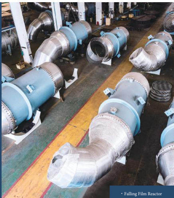
• Falling Film Reactor
